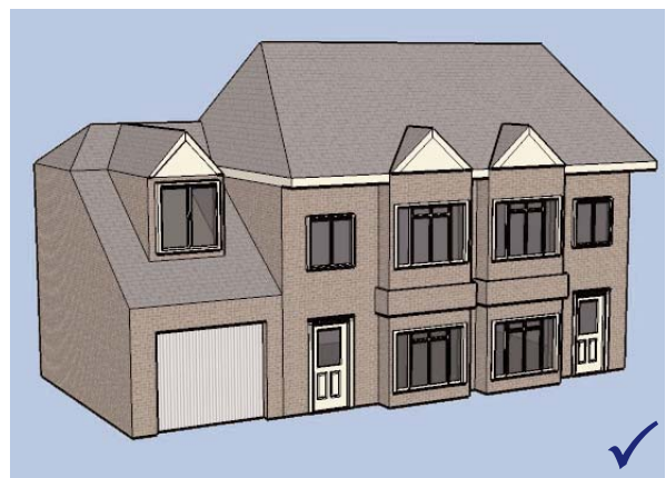
An alternative to the above shows a sloping roof and dormer window.
