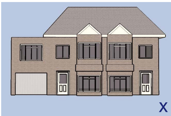
An unacceptable extension which can lead to a terracing effect .
