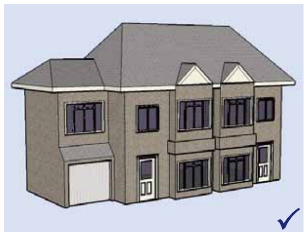
A typical design solution which is subservient to the original house. The extension is set back from the front building line of the original house.
