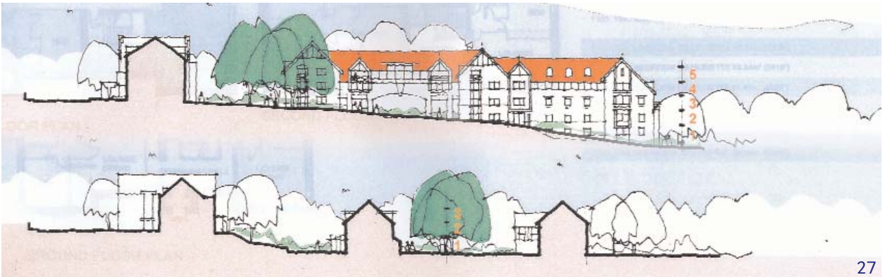
Simple and legible cross sections show how the proposed development responds to the site topography and how it relates to existing buildings in and around the site.
