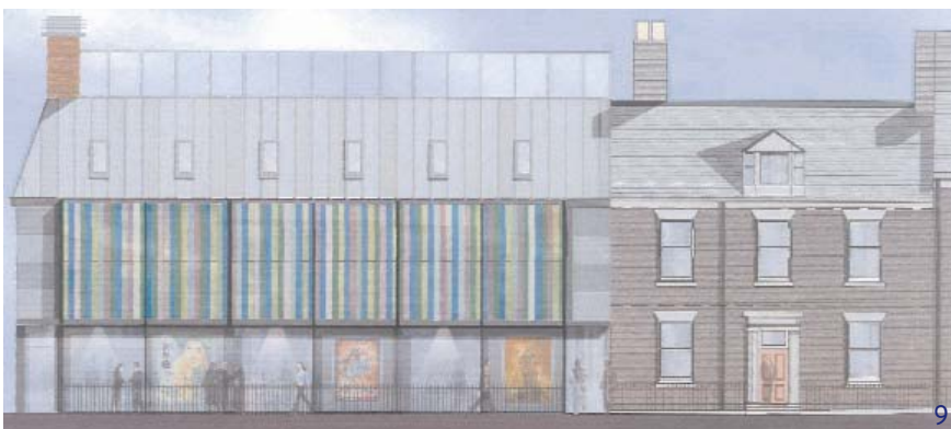
The Place, Sunnyside - high quality contemporary architecture alongside a listed property. The new building respects the scale and proportions of the historic properties and complements the established building materials with the use of coloured glazed louvres.
