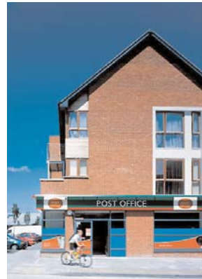
Oakridge village, Basingstoke - high levels of natural surveillance have been achieved throughout the development. Parking and the area of open space are overlooked and windows on gable ends provide surveillance to the shop.
