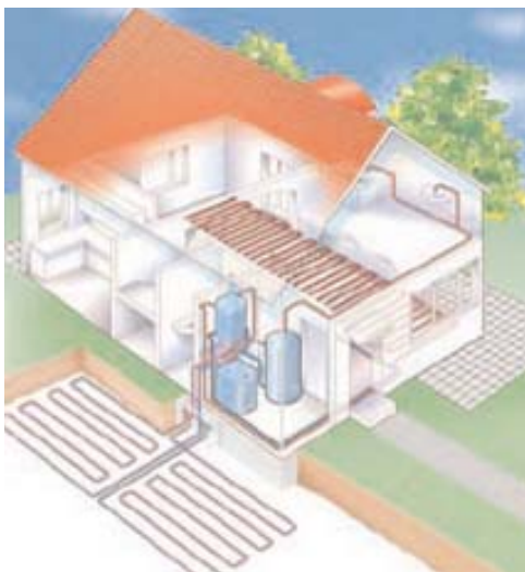
Ground-Source Heat Pump System
