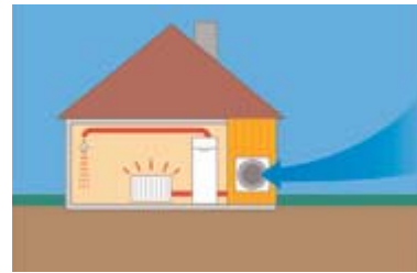
Air-source heat pump
