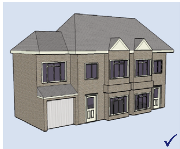
A first floor extension above an existing garage. The new first floor extension is subservient to the main house.
