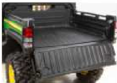
Tailgate lowered to 150 degrees Deluxe cargo box tilt
