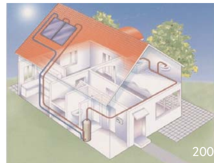
Solar thermal hot water system
