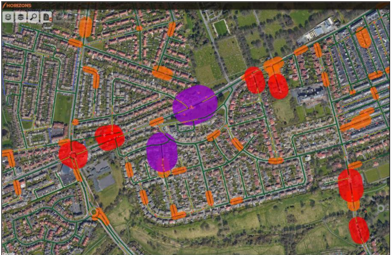
Figure 3 – defect cluster analysis in Horizons Asset Management Software
